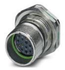
Device connector for rear wall, straight, shielded: yes, SPEEDCON locking, M23, No. of pos.: 16+2+PE, type of contact: Socket, Crimp connection, Axial seal, Central fixing
