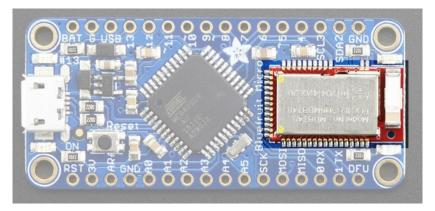
Finally there's the BLE module. This is the radio-handling part. It is an FCC/CE-certified emittermodule with a ceramic antenna. The ATmega32u4 talks to this module over SPI using our Arduino library to transmit and receive data. It is based on the nRF51822 chipset from Nordic Semiconductor.
