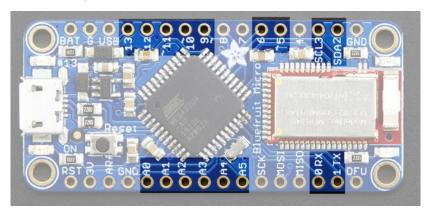
All of these pins are digital input/output pins, with 3.3V logic. Some have extra capabilities
