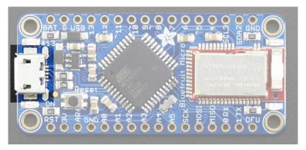
Starting from the left, there's the Micro USB connector. This is how you power and program the Bluefruit Micro. If you added on the LiPoly backpack you can also recharge the battery this way.
