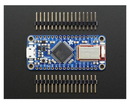
Each order comes with one fully assembled and tested Bluefruit LE Micro board. The ATmega32u4 on board comes with a USB bootloader for quick programming. The BLE module comes with our latest firmware. We also include some headers which you can solder in to use the module in a solderless breadboard.
