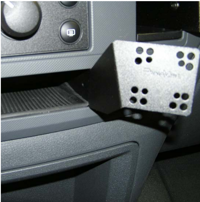
InDash Installed Showing Location
