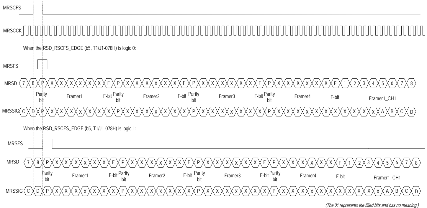
Figure 34. T1/J1 Receive Multiplexed Mode - Functional Timing Example 2
