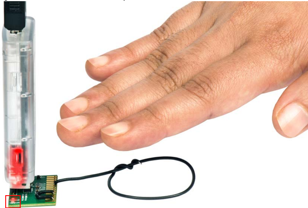
Figure 3-13. LED Glows on Proximity Detection
