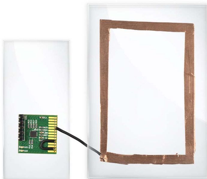
Figure 3-2. A Proximity Sensor Implementation Using a Wire Loop
