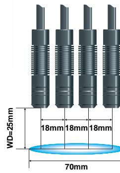
When high-intensity heads equipped with ANUJ6475S (cylindrical lens) are used with 18 mm pitches as shown in the figure, an entire linear area of approx. 70 mm wide can be reliably irradiated at 350 mW/cm<sup>2</sup> or higher intensity.
