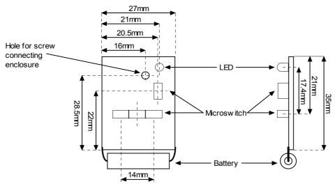
RF Solutions microswitch has a lead pitch of 6.35mm and a height of 4mm
