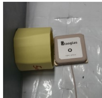
Ground side of antenna
