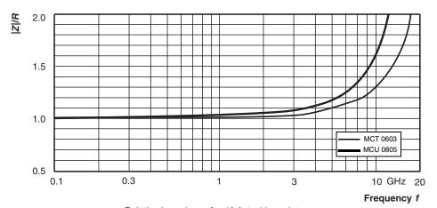
Relative impedance for 49.9  $\Omega$  chip resistor
