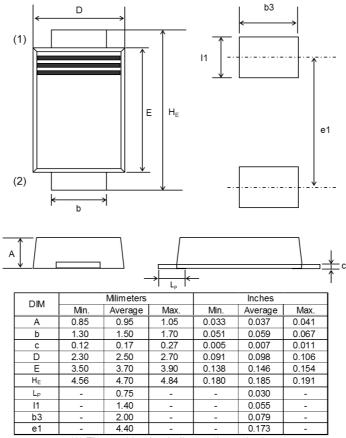
(1) The marking bar indicates the cathode.(2) The direction indicates the anode.
