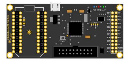
This is a FT2232H based JTAG programmer shield that is compatible with OpenOCD and Broadcom's WICED IDE. The FT2232 chip is setup to provide an USB-JTAG and USB-UART interface simultaneously. The FT2232 can be also reconfigured by the user by reprogramming the on-board config EEPROM. The unused pins are clearly marked and broken out into easy to access header holes.
