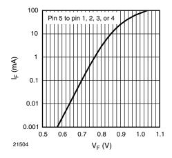
Fig. 4 - Typical Forward Current I<sub>F</sub> vs. Forward Voltage V<sub>F</sub>
